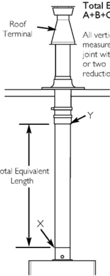
All vertical and angled runs must be included, measured from the boiler adaptor (point X) to the joint with the flue terminal (point Y). One  $93^\circ$  bend or two  $135^\circ$  bends can be included without reduction of the flue length.
