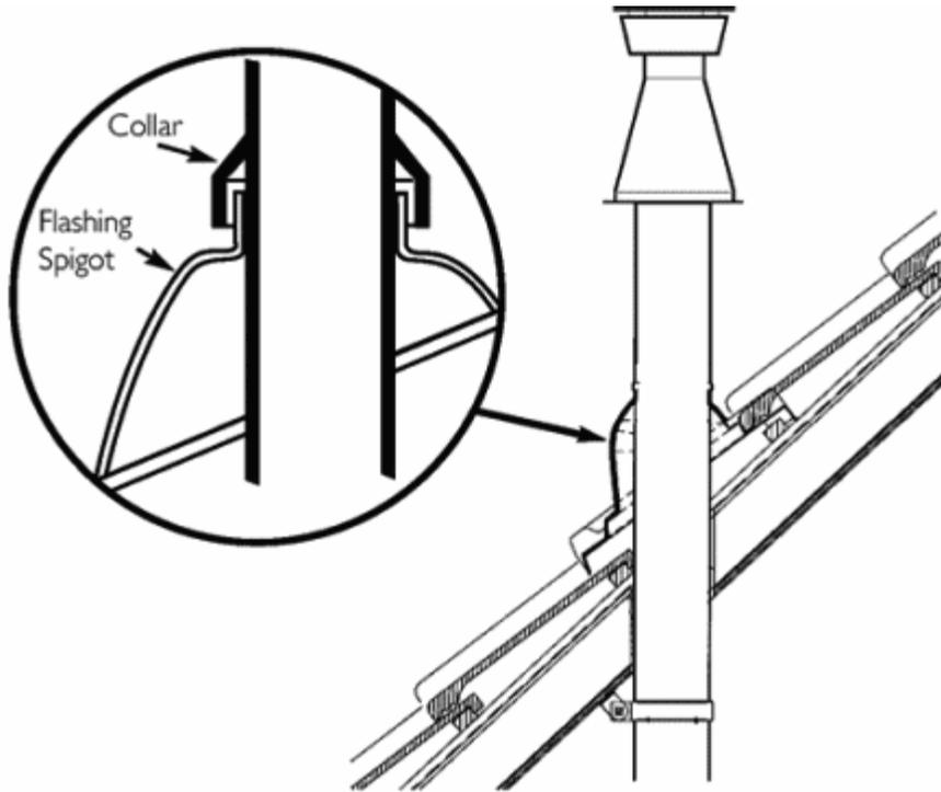
**It is necessary to cut the flue terminal air duct by 170mm. Dimensions x & y must be 60mm.**
