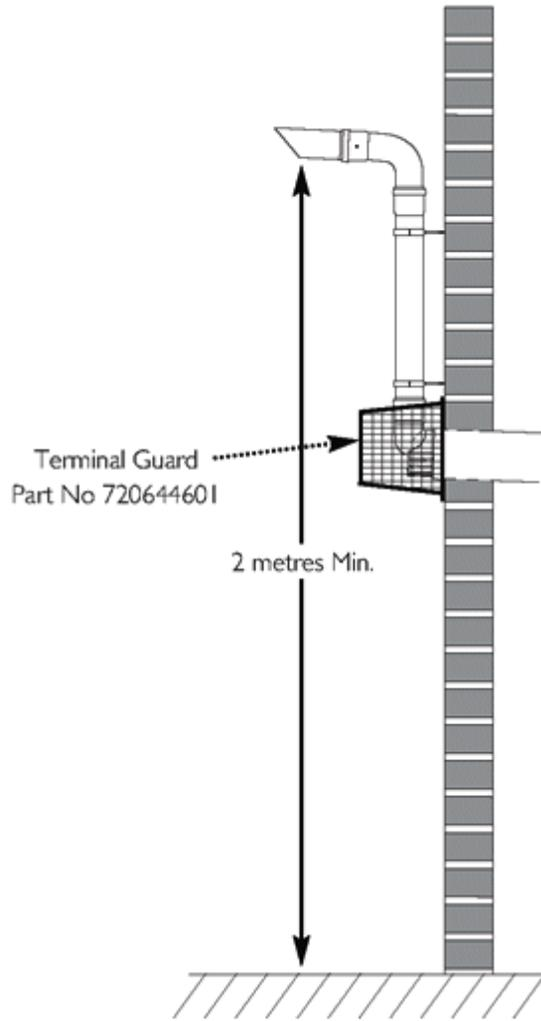
The outlet of the PDK **MUST** be at least 2 metres above ground or balcony level. If necessary additional 60 Ø extensions should be used to achieve this.
