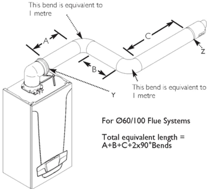
The **MAXIMUM** total equivalent length is stated in the Installation & Servicing Instructions supplied with each boiler.
