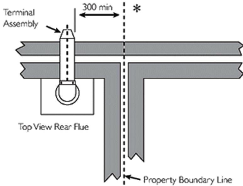
\* Reduction to the boundary is possible down to 25mm but flue deflector part no. 5111068 must be used.
