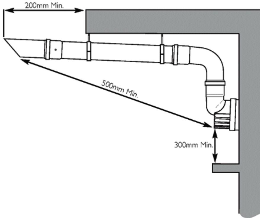
The inlet of the PDK **MUST** be at least 300mm above ground or balcony level or any projection or ledge. A guard must be fitted where the inlet is below 2 metres.
